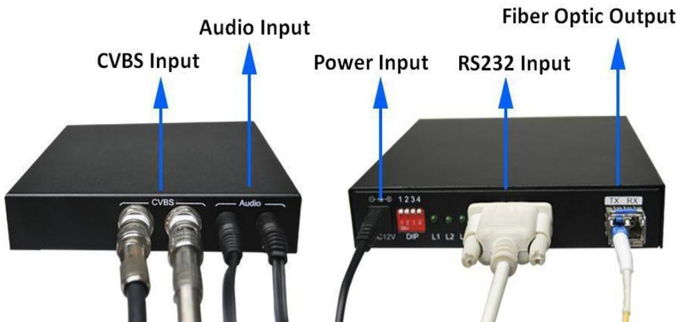
Note: Please connect one single-mode optical fiber to the **TX** port in the fiber optic connector.
